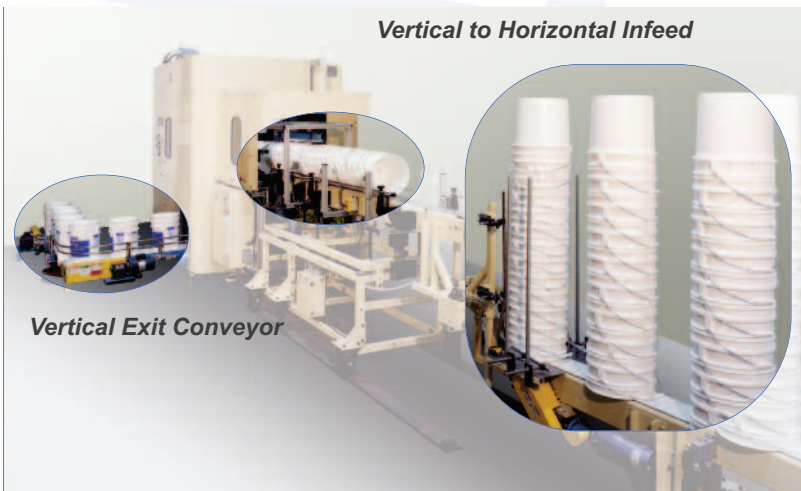
Vertical to Horizontal Infeed and Vertical Exit Conveyor
